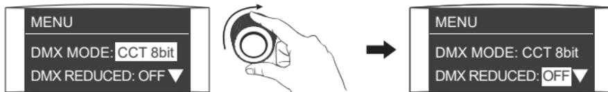
Rotate the right knob to DMX REDUCED CHANNELS.
