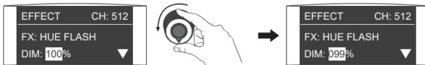
Rotate the left knob to set the corresponding parameters.
