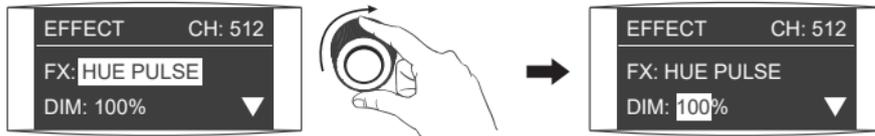
Rotate the right knob to select DIM, HUE, SAT or PULSES/MIN.
