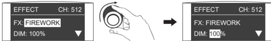
Rotate the right knob to select DIM, COLOR, SPEED or DECAY.
