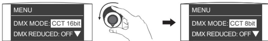
Rotate the left knob to select the desired DMX mode.
