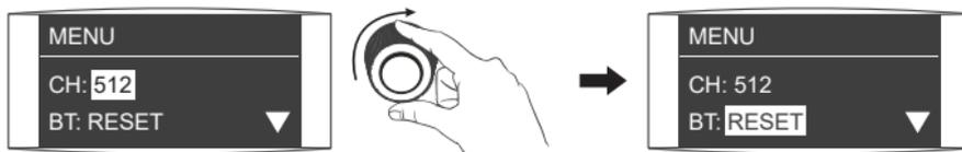
Rotate the right knob to select CHANNEL, BLUETOOTH, DMX MODE, DMX REDUCED CHANNELS, DMX DIMMING CURVE, DMX SMOOTHING, CRMX, WIRELESS PROTOCOL, FAN, FIRMWARE UPDATE, LANGUAGE or VERSION.
