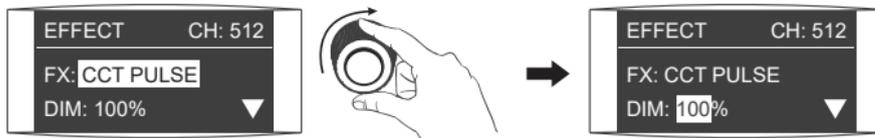
Rotate the right knob to select DIM, CCT, G/M or PULSES/MIN.
