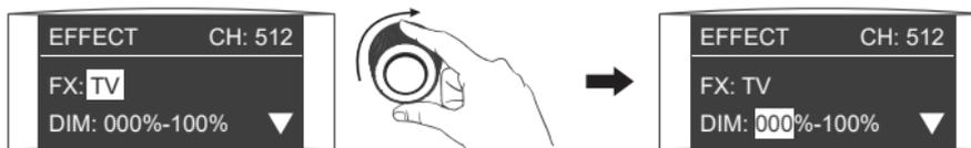
Rotate the right knob to select DIM, CCT, G/M or SPEED.
