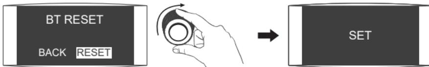
Rotate the right knob to RESET, and press the right knob to set.
