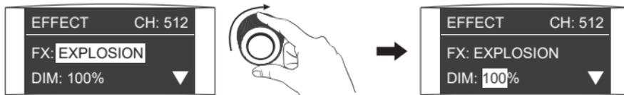
Rotate the right knob to select DIM, CCT, G/M, SPEED or DECAY.
