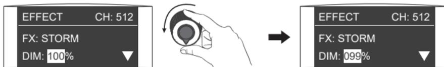
Rotate the left knob to set the corresponding parameters.
