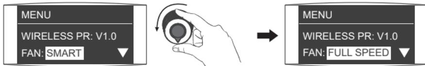
Rotate the left knob to select SMART, FULL SPEED, LOW SPEED or OFF.
