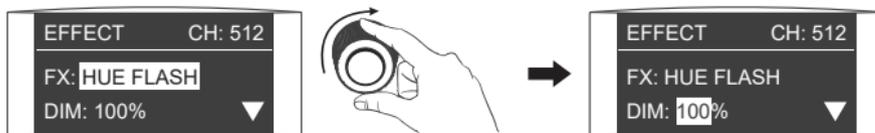
Rotate the right knob to select DIM, HUE, SAT or INTERVALS.
