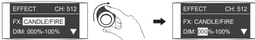
Rotate the right knob to select DIM, CCT, G/M or SPEED.
