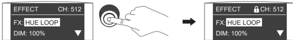
Long press the right knob to lock the lighting parameters. The current settings cannot be changed by pressing the button or rotating the knobs.
