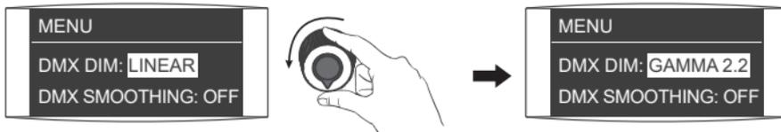
Rotate the left knob to select the desired dimming curve.
