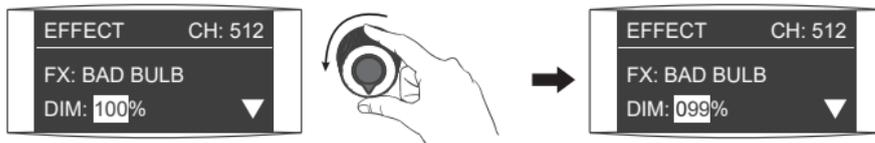
Rotate the left knob to set the corresponding parameters.
