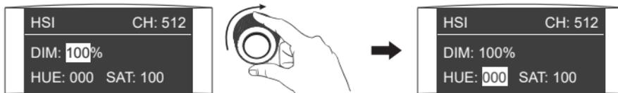
Rotate the right knob to select DIM, HUE or SAT.
