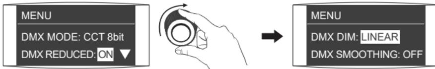
Rotate the right knob to DMX DIMMING CURVE.
