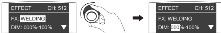
Rotate the right knob to select DIM, CCT, G/M, SPEED or PAUSE.
