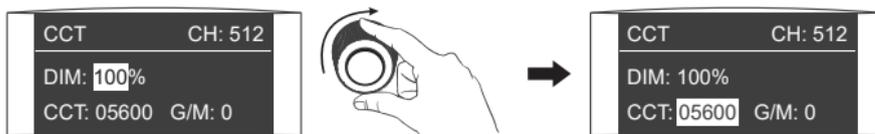
Rotate the right knob to select the DIM, CCT or G/M.
