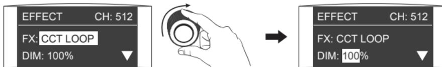
Rotate the right knob to select DIM, CCT or SPEED.
