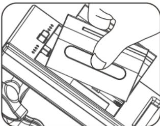
Mount two NP-F batteries onto the battery holder of the grip.
